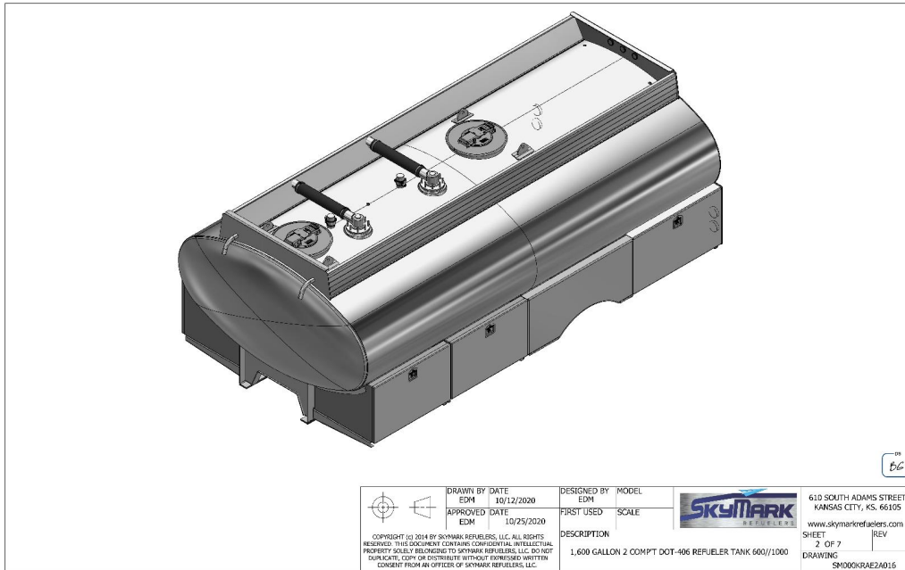
Figure 14 Booster MFOD 1,600 Gallon Capacity Tanks (Two Compartment Refueler Tank (Oblique View Left Side))
