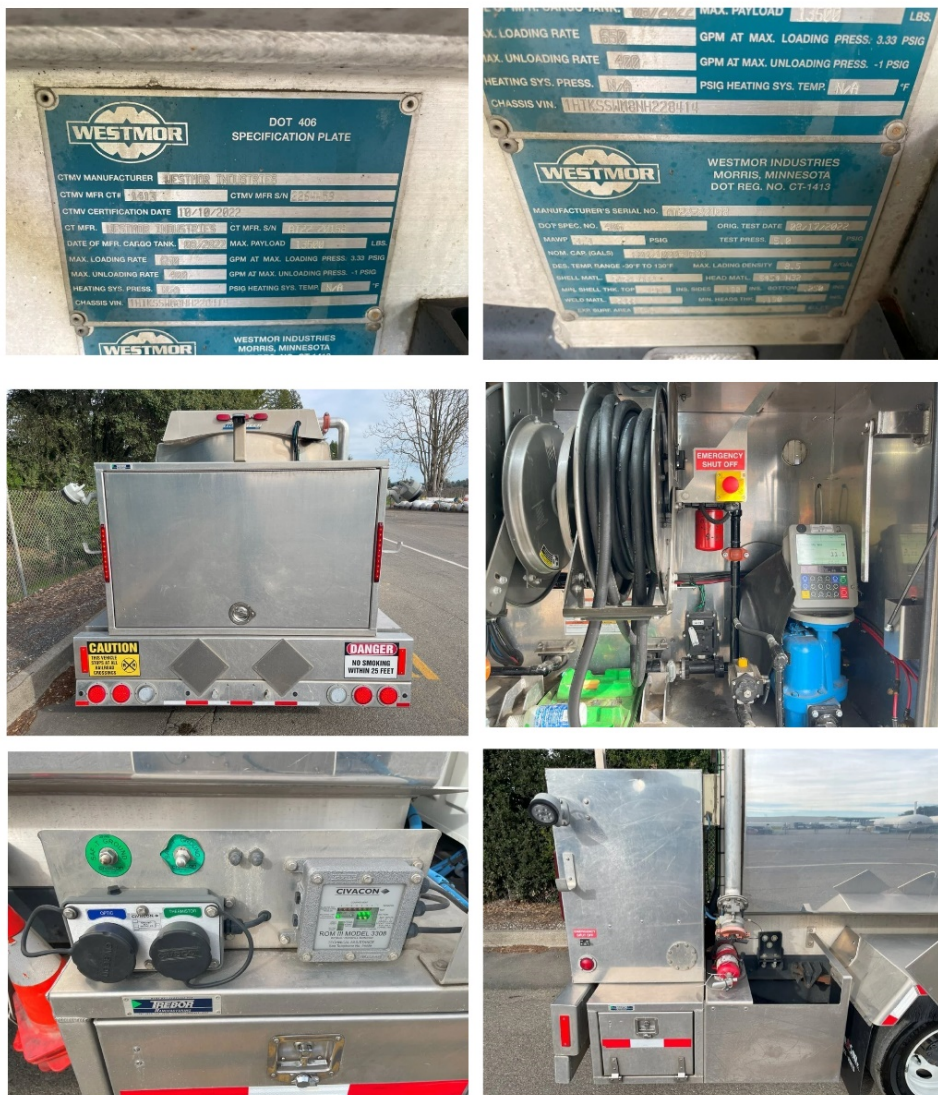
Figure 8 Booster MFOD With 1,600 Gallon Capacity Tanks (Additional Photos)
